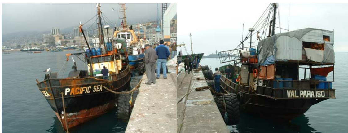
Fig. A2.15. Bow (left) and stern views of an industrial swordfish longline vessel in the port of Valparaiso.
