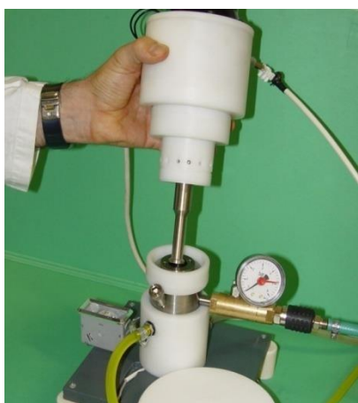
Figure 2b. Horn and reaction chamber of the same reactor.
