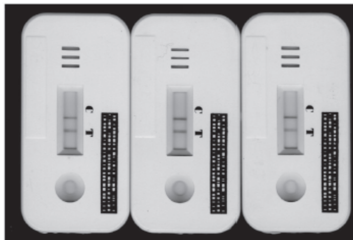
Figure 1. Image of lateral flow devices used for measuring aflatoxins in three maize samples, naturally contaminated at three levels. Concentrations of aflatoxins (obtained by the LC-FLD method) from left to right: not detectable (negative sample), 5.4 \mu\text{g kg}^{-1} (low contamination level, close to EU MRL (European Commission 2003)), and 17.1 \mu\text{g kg}^{-1} (high contamination level).
