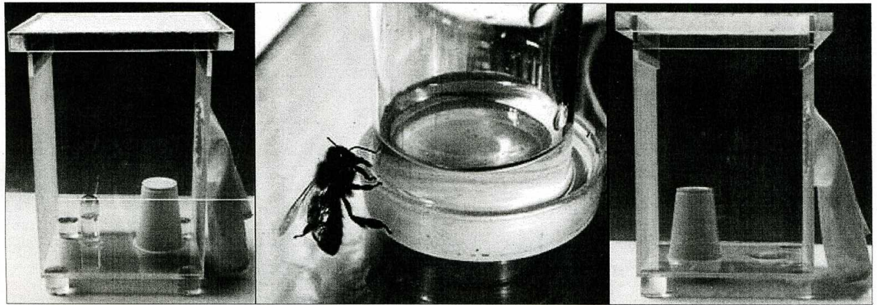
Fig. I – Cage prepared for the ingestion trials (left); detail of the feeder pointing out the narrow space where the bees can feed (centre); after 1 hour the feeder is covered and the bees can feed on some candy (right).
