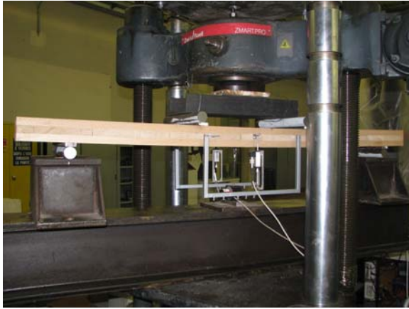
Figure 7. 4-points bending test equipment.
