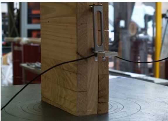
Figure 9. Particular of strain gage used for compression test (chestnut).
