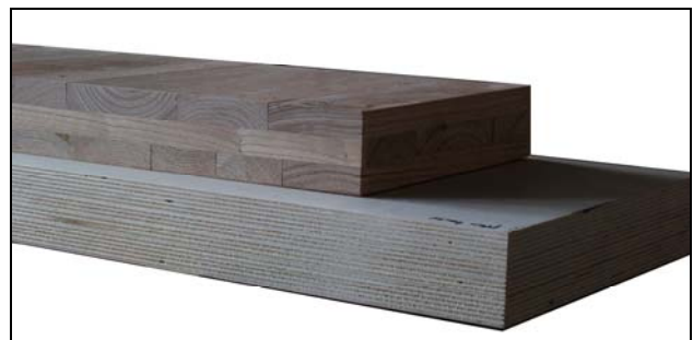
Figure 6. Chestnut and poplar specimens of the X-Lam type produced with local wood.
