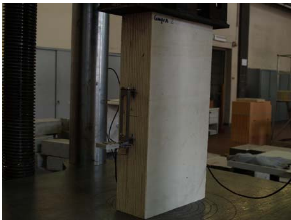
Figure 8. Compression test equipment (poplar.)
