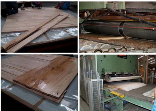
Figure 4. Chestnut panel during gluing and pressing.
