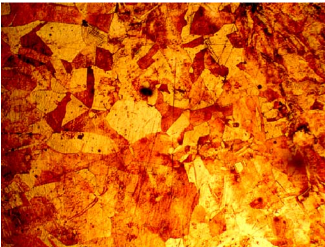
FIGURE 5 Photomicrograph (x80) of the body of the Savignano 994 sample showing a regular grain distribution characterized by twin lines typical of recrystallisation
