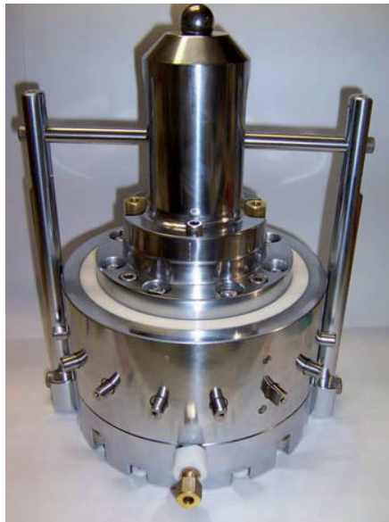
Fig. 1. Oedometer ERT cell used in the investigation.
