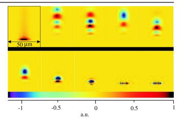
FIG. 3 (color online). (Top left) Map of the damage produced by the ion beam in terms of vacancy density. (Rest of the figure) In the same spatial scale, amplitude maps of nine simulated modes propagating in the waveguide irradiated at a fluence of  $2 \times 10^{16}$  cm<sup>-2</sup>.
