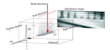
FIG. 1 (color online). Scheme of the implantation geometry. (a) Vacancy density distribution as a function of depth z. (b) The same distribution in a gray-scale representation, as a function of y and z. (c) Simulation of the defect positions along the buried microchannels. (d) Interference pattern produced by the implantation.
