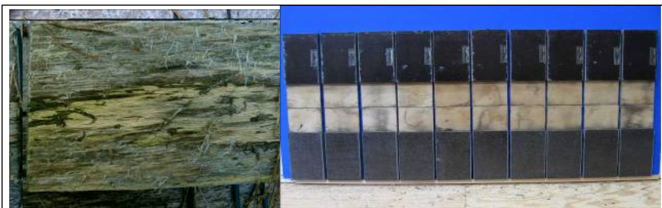
Figure: Lap joint samples after 1.5 years exposure (intensive decay in Poplar plywood C2; any decay in coated birch K3)
