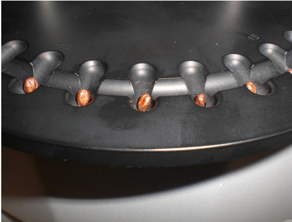
FIGURE 1. Positioning of intact berry seeds on the Solids Transmittance modules of the NIR-Flex N500 spectrophotometer.
