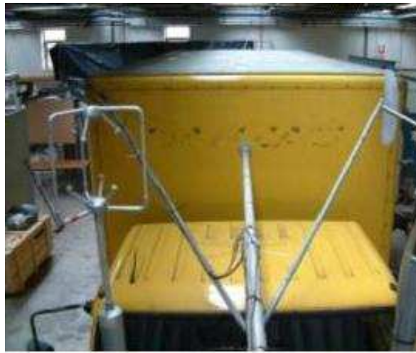
Figure 6: Front view. Front tapping points, anemometer
