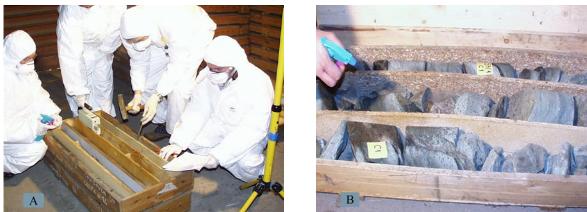
Fig. 4 Drill core sampling operation (a). Due to the possible dispersion of asbestos fibers during the operations, effective measures are necessary to prevent the laboratory pollution and the risk of exposure of the operators (b).
