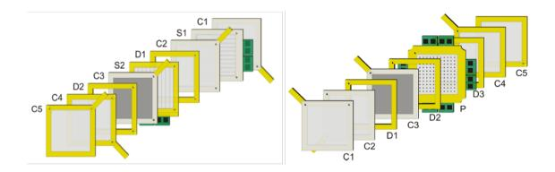
Figure 1: schematic drawing of the detector assembly of BOX1 (left) and BOX2 (right): S1 and S2 are the anodes segmented in strips, P is the anode segmented in pixels, C3 is the anode of the integral chambers, C2 and C4 are the cathodes. The frames D1, D2 and D3 are needed to provide the desired gap between electrodes while C1 and C5 are added to provide an additional gas gap on both sides of the assembly, as explained in the text.
