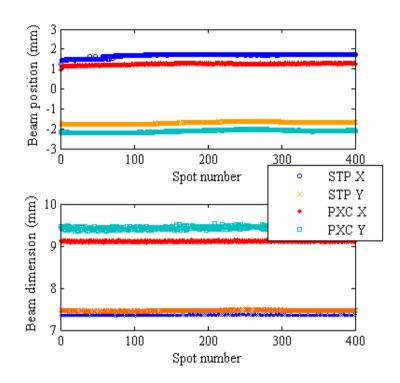
Figure 7: beam position and beam FWHM measured with the strip and pixel chambers in a run with 400 identical spots.
