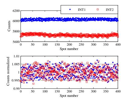
Figure 6: number of counts as a function of the spot number for the integral chambers (top) and the same quantity normalized to the average (bottom). The dashed lines correspond to the  $\pm 0.5\%$  deviation from the average.
