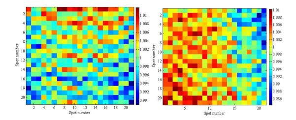
Figure 9: uniformity of the two integral chambers measured in a 21x21 grid of points covering an area of  $100x100 \text{ mm}^2$ . The number of counts in each point of the grid normalized to the average number of counts over all the points of the grid, is shown.
