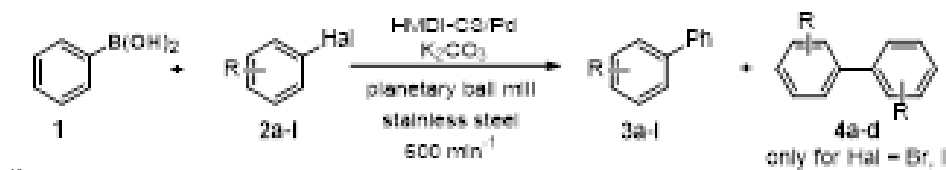
Scheme 1. Suzuki cross-coupling reaction of aryl halides in a planetary ball mill (cf. Tab. 1).
