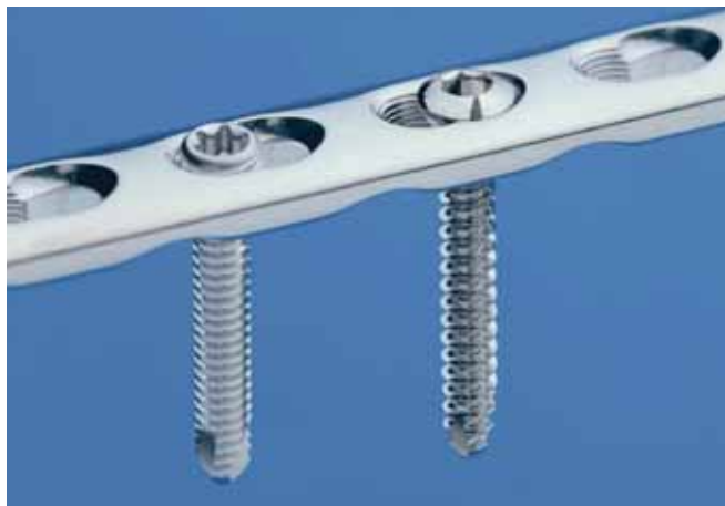
FIGURA 1 - Foro combi-hole : vite bloccata LHS ( Locking Head Screw ) a sinistra; vite corticale CS ( Cortical Screw ) a destra.
