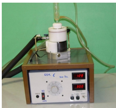
Figure 1. A high-power 300 kHz US-reactor with cooling system.
