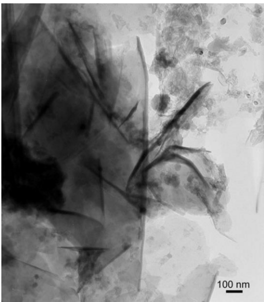
Fig. 7. Transmission electron micrograph of chrysotile layers via curling formed on the edge of forsterite relict, from run D5 (360°C, 100 MPa, 160 h), reactant d = glass (2) + H 2 O.
