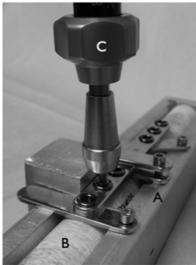
Figure 2 Jig used for specimen preparation. The custom made jig (A) secures the plate (in this case Fixin) at a 2 mm distance from the bone model (B). The screw is inserted using a torque limiting device (C).
