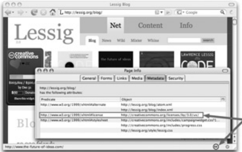
Figure 9: The MozCC Mozilla Add-On. The status bar shows a CC icon that indicates to the user that the page is CC-licensed. A click on the icon reveals the detailed metadata in a separate window.
