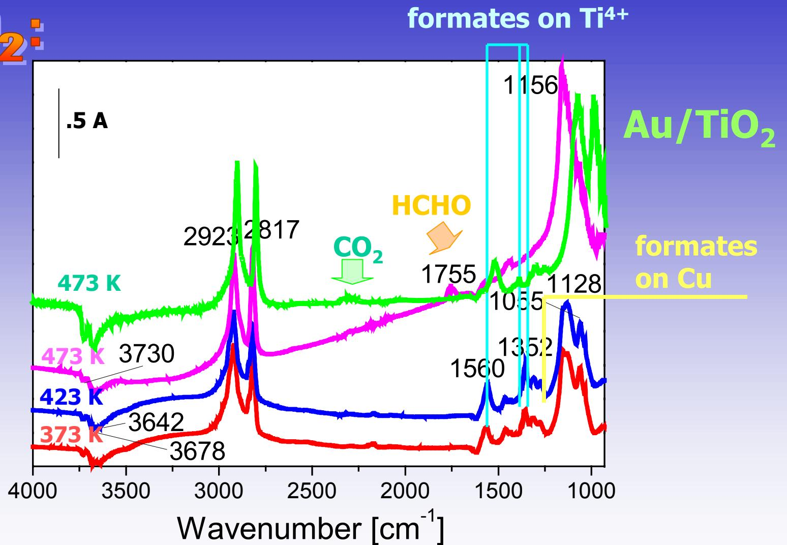
✓  $\text{CH}_3\text{OH}-\text{H}_2\text{O}-\text{O}_2$  interaction at increasing temperature:
