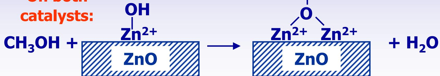
✓ **CH<sub>3</sub>OH interaction at increasing temperature:**
