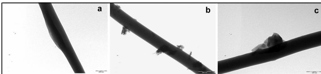
Figure 8. Transmission electron microscopy of electrospun M-1 mat showing GO flakes deposited b) on the surface or a,c) partially embedded into gelatin fibers. Scale bar: 200 nm a,c); 500 nm b).
