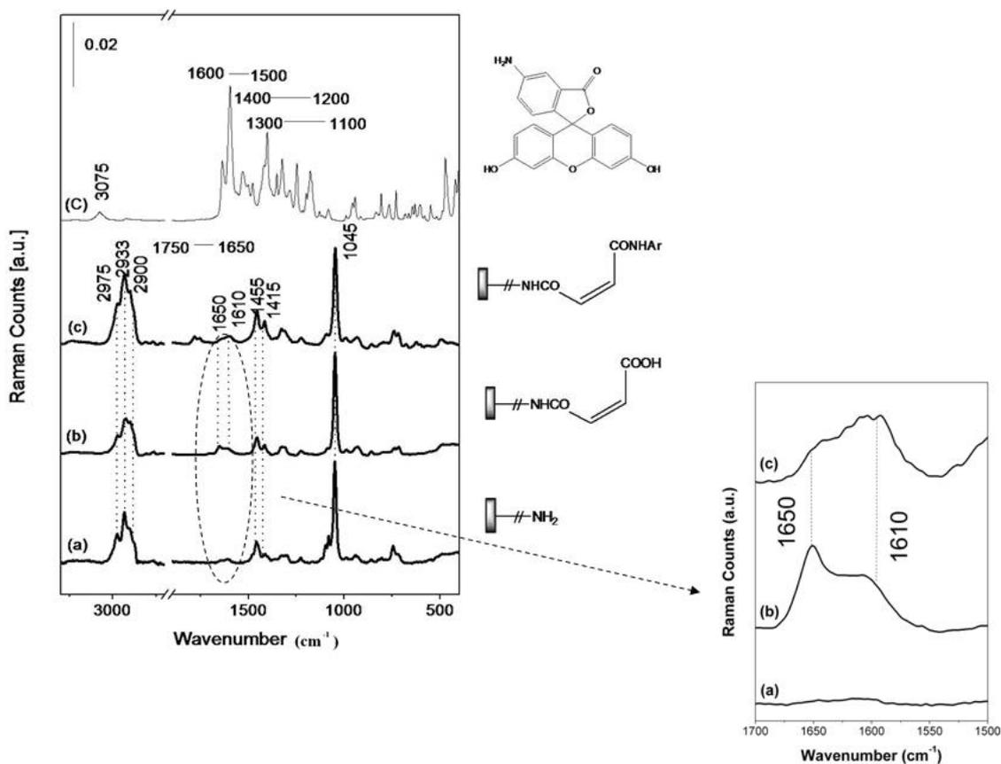
**Figure 3.** Raman spectra in the 3300-400  $\text{cm}^{-1}$  spectral range carried out on: (a) as-synthesized samples (APTES-SG); (b) ~~APTS25SG423~~ APTES-SG after functionalization with N-(5-Fluoresceinyl)maleamic acid (APTES-SG-MAAF). As reference, the spectrum of N-(5-Fluoresceinyl)maleamic acid (MAAF) is reported (see spectrum D). **Blown-up in the 1700-1500  $\text{cm}^{-1}$  spectral range.**
