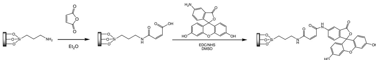
**Scheme 2.** Synthesis of N-(5-Fluoresceinyl)maleamic acid and conjugation to **APTES-SG**. **APTS25SG423**.
