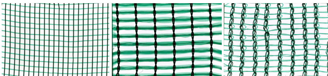
Fig. 1 – Italian texture (left), English texture (center), Raschel texture (right). (Modified from Castellano et al. , 2008).
