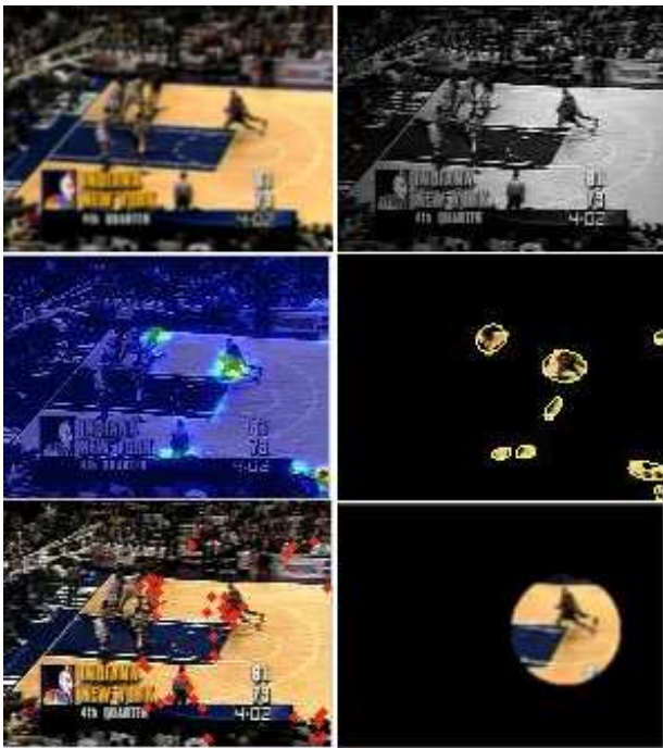
Fig. 2. The Ecological Sampling implementation at a glance. From top to bottom, left to right: the original frame; the foveated frame; the raw saliency map; detected patches; sampled interest points; the sampled FOA
