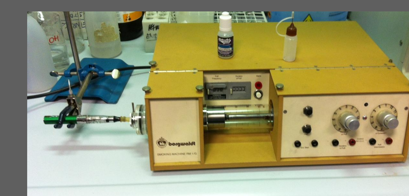
Figure 4: Smoking machine generating aerosol from e-cigarette
