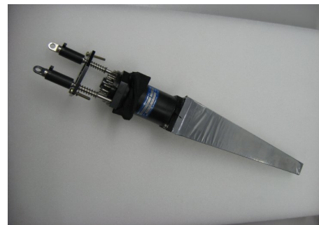
Figure 3. BGO crystal coupled to the photomultiplier.
