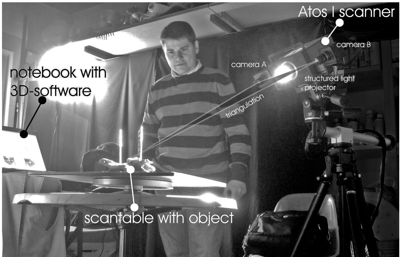
Fig 1: Scan setting with the structured light scanner ATOS 1 from GOM. The scanner uses a single light source to project various light patterns on the object. Two cameras record the object and a software calculates the 3D matrix of the object by triangulation. For the specimen SMA 0004 30 scans from different directions per vertebrae were necessary in order to create the point cloud for the digital model.
