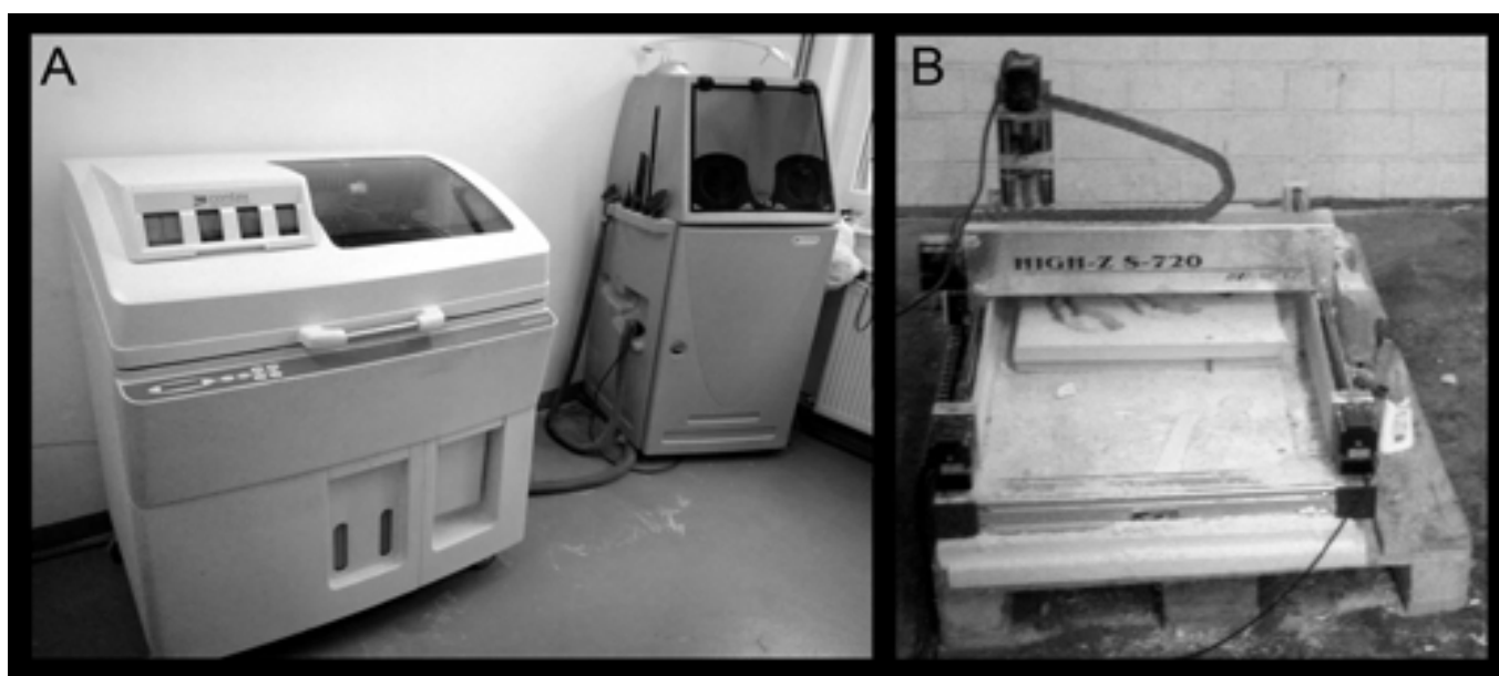
Fig 3: Hardware used to reproduce the digital objects. A: Zprint 510 from Z corp. Build size 254 x 356 x 203 mm, layer size 0.08 to 0.2mm, equipment dimensions 107 x 79 x 127 cm, weight 204kg. In the background the air cleaning station can be seen.
