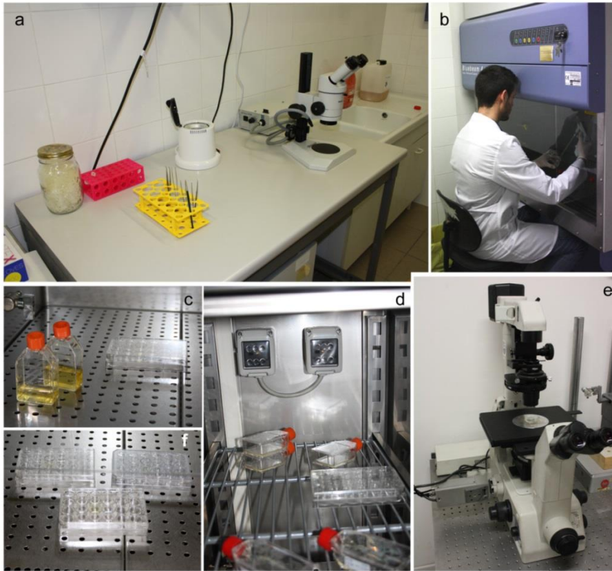
Figure 1. Minimal equipment needed consists of a table or bench that can be cleaned with ethanol solutions for the performance of dissections at the stereomicroscope (a), a laminar flow hood (or biological safety cabinet) to manage cells and sterile reagents (b), a refrigerated incubator to maintain cell flasks/dishes at 24-28°C (c, d) and an inverted phase contrast microscope to observe cells (with a 10X or 20X, and 40X phase contrast objectives) (e).
