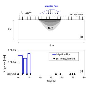
Figure 2: Schematic representation of the system geometry (a) and time-behavior of the infiltration flux rates imposed at the surface boundary (b). Black dots indicate the time of ERT measurements.
