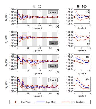
Figure 8: Heterogeneous test case results: comparison of the iterative approach (N=20) with a non-iterative simulation with ensemble size N=160. The convergence of the four hydraulic conductivities for the iterative (panels a,c,e,g) and non-iterative (panels b,d,f,h) cases is illustrated (runs with  $\sigma_{\Phi}=20\%$  and randomly perturbed measurements).
