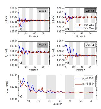
Figure 7: Heterogeneous test case results: convergence of the hydraulic conductivities (ensemble mean values) of the four zones (a-d) and mean RMSE (e) for different initial values  $\mu_{\lambda_0}$ . The results are relative to  $\sigma_{\Phi}=5\%$  with randomly perturbed measurements.
