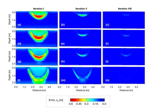
Figure 5: Spatial distribution of the error  $\epsilon_{\psi}$ , representing the discrepancy between simulated (ensemble mean) and true system state (pressure field).
