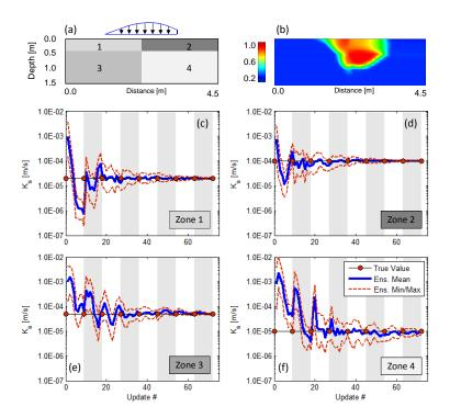
Figure 6: Heterogeneous test case results: (a) conceptual model of the model domain (divided into 4 zones with different soil properties) and (b) the simulated soil saturation at t=5.5h. Convergence of the hydraulic conductivities of the four zones is shown in panels c-f. The results are relative to  $\sigma_{\Phi}=5\%$  with randomly perturbed measurements.
