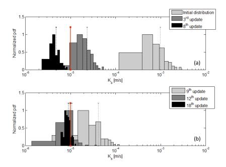
Figure 4: Synthetic test case results: pdf of the hydraulic conductivity normalized on the maximum value of the pdf. Panel (a) and (b) refer to the first and second external iteration of the SIR method, respectively. The simulation was run with an ensemble size N=100. Dotted lines indicate the ensemble mean and the red line indicates the true value of  $K_s$ .
