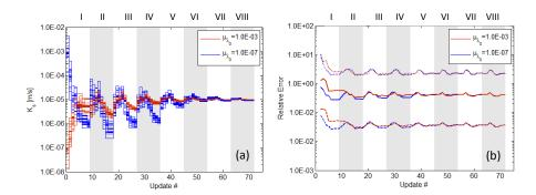
Figure 9: Field experiment results: convergence of the hydraulic conductivity (a) and relative errors (b) for different initial values of hydraulic conductivity  $\mu_{\lambda_0}$ . The roman numerals at the top of the panels indicate the external iteration count. Mean relative error  $(\epsilon_y)$ , Mean  $RMSE_y$  and Maximum Relative error  $(\epsilon_{y,max})$  are shown.
