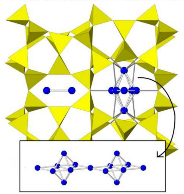
Water molecules intruded in Si-FER compressed in m.e.w.
