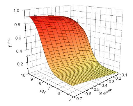
**Figure 7.** Fraction of triclosan transformation accounted for by direct photolysis, as a function of pH and  $\Phi_{triclosan}$ . Other water conditions: 0.1 mM nitrate, 1  $\mu$ M nitrite, 1 mM bicarbonate, 30  $\mu$ M carbonate, 5 mg C L<sup>-1</sup> DOC, 5 m depth.
