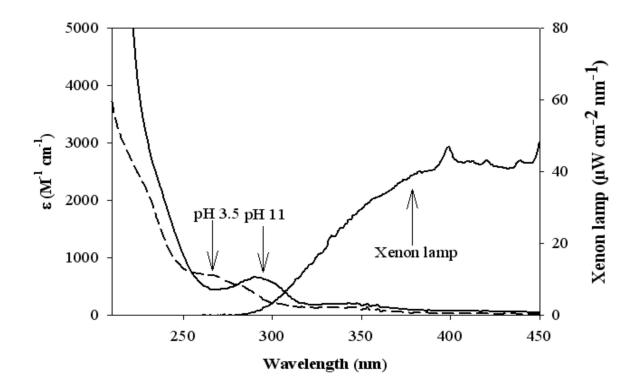
**Figure1.** UV-vis absorption spectra of triclosan at pH 3.5 (Htric) and 11 (Tric<sup>-</sup>) (molar absorption coefficient ε). Emission spectrum of the xenon lamp (irradiance on top of the solutions).
