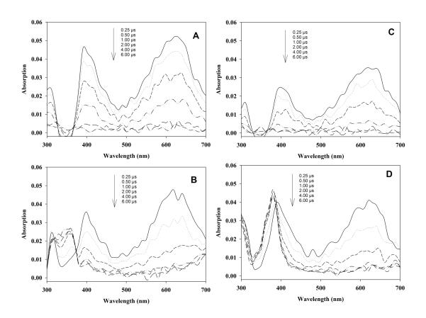
**Figure 2.** Transient absorption spectra obtained after 355 nm excitation of  $5 \times 10^{-5}$  M 1NN, in pure water at pH 3.5 (**A**) and 9.5 (**C**), and in the presence of triclosan  $(1.5 \times 10^{-4} \text{ M})$  at pH 3.5 (**B**) and 9.5 (**D**). In all the experiments the temperature was  $295 \pm 2$  K.
