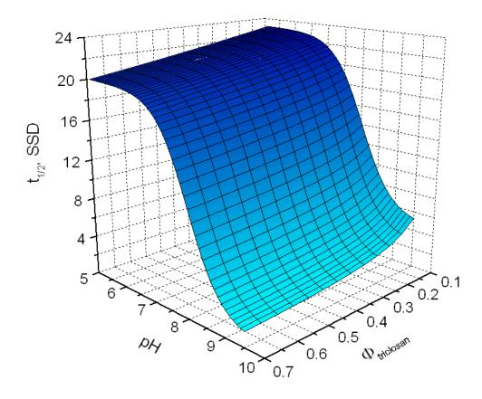
**Figure 6.** Half-life time of triclosan, as a function of pH and of the direct photolysis quantum yield  $\Phi_{triclosan}$ . Other water conditions: 0.1 mM nitrate, 1  $\mu$ M nitrite, 1 mM bicarbonate, 30  $\mu$ M carbonate, 5 mg C L<sup>-1</sup> DOC, 5 m depth.
