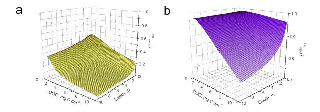
**Figure 5.** Fractions of the overall transformation accounted for by direct photolysis, for both HTric (a) and Tric<sup>-</sup> (b), as a function of water depth and DOC. Other water conditions: 0.1 mM nitrate, 1  $\mu$ M nitrite, 1 mM bicarbonate, 30  $\mu$ M carbonate;  $\Phi_{triclosan} = 0.4$ .
