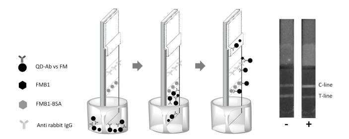
Graphical abstract. The fluorescent immunochromatographic strip test based on the use of Quantum Dots as labels for the sensitive and rapid detection of fumonisins (FMs) in maize flour. The test allows the rapid and simple visual detection of FM contaminations and the quantitative determination of FMs at levels of regulatory interest.
