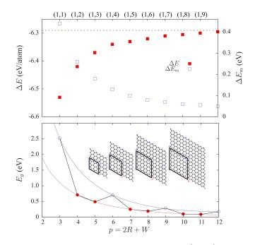
Figure 2: (color online) Energetic and electronic properties of (1, W) BNG structures as a function of p = 2R + W. Upper panel: cohesive energy  $\Delta E$  (the graphene,  $p \to \infty$ , limit is given by the horizontal line) and energy of mixing  $\Delta E_m$  (zero by definition at p=0 and  $p=\infty$ ). Lower panel: evolution of the electronic band gap  $E_g$ ; red and blue lines are just meant as eye-guides. The inset shows the structure of (1, W) BNG configurations as p increases.
