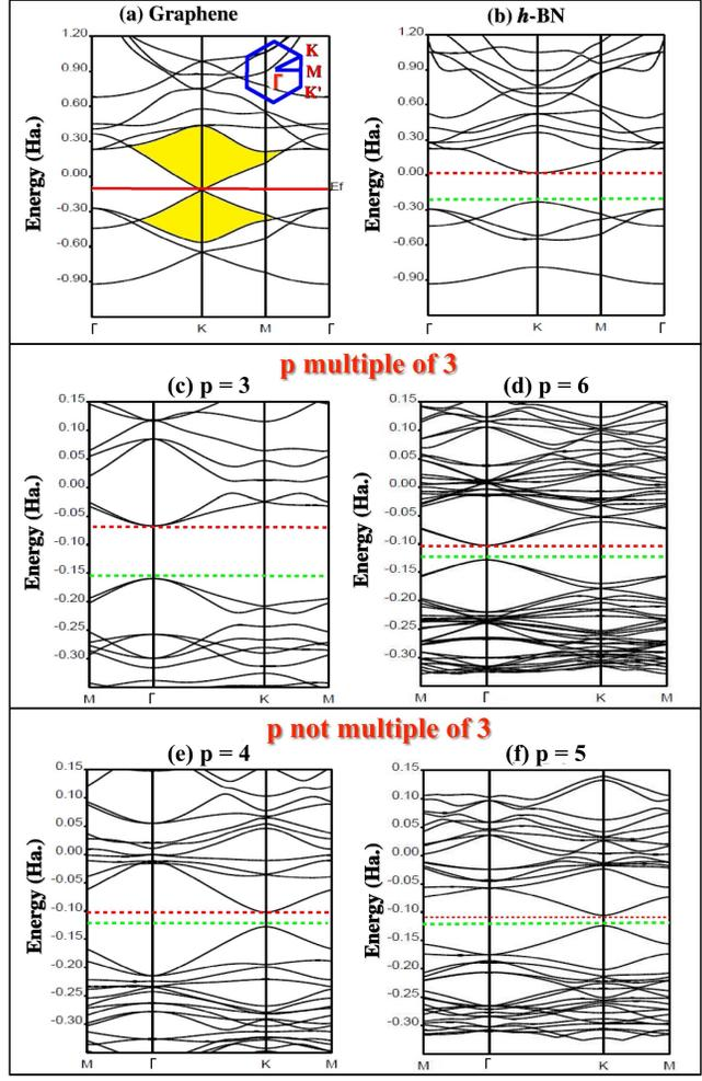
Figure 3: (color online) Energy band structure of (a) pristine graphene, (b) pristine  $h$ -BN, (c-d) BNG  $(1, W)$  structures with  $p$  multiple of 3, (e-f) BNG  $(1, W)$  structures with  $p$  not multiple of 3. HOCO and LUCO energy levels are drawn as dashed green and red lines, respectively.
