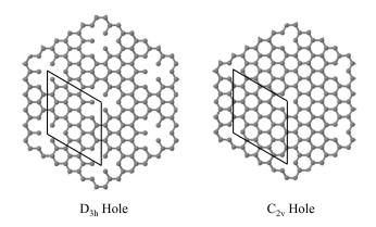
Figure 5: (color online) Graphical representation of the structure of two defects, one of  $D_{3h}$  and one of  $C_{2\nu}$  point-symmetry, of graphene (holes in this case) that break its inversion symmetry. The unit cell of the *p*=4 case is sketched in both cases with black continuous lines.
