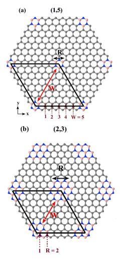
Figure 1: (color online) BN-doped piezoelectric graphene in different configurations (R, W). The radius *R* of BN rings and the wall width *W* separating them are graphically defined. The unit cell of each configuration is shown as thick black lines.
