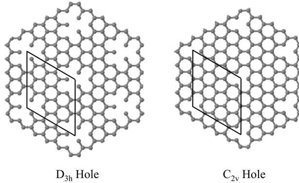
Figure 5: (color online) Graphical representation of the structure of two defects, one of  $D_{3h}$  and one of  $C_{2v}$  point-symmetry, of graphene (holes in this case) that break its inversion symmetry. The unit cell of the  $p=4$  case is sketched in both cases with black continuous lines.
