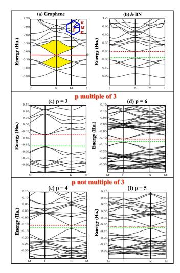
Figure 3: (color online) Energy band structure of (a) pristine graphene, (b) pristine *h*-BN, (c-d) BNG (1, W) structures with *p* multiple of 3, (e-f) BNG (1, W) structures with *p* not multiple of 3. HOCO and LUCO energy levels are drawn as dashed green and red lines, respectively.
