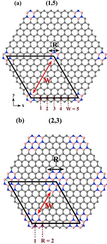
Figure 1: (color online) BN-doped piezoelectric graphene in different configurations  $(R, W)$ . The radius  $R$  of BN rings and the wall width  $W$  separating them are graphically defined. The unit cell of each configuration is shown as thick black lines.
