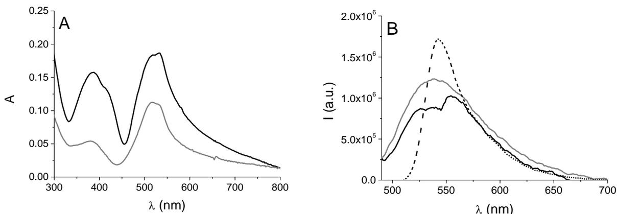
**Figure 3.** A) Absorption spectra of **1** (black) and **2** (grey) in culture medium. B) Fluorescence emission spectra ( $\lambda_{\text{exc}}=480$  nm) of optically matched solutions of **1** (black) and **2** (grey) in culture medium and, for comparison, **1** in acetonitrile (dashed).
