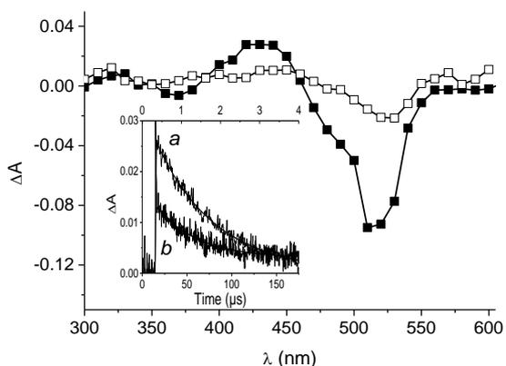
**Figure 4.** Transient absorption spectra observed 0.1  $\mu\text{s}$  after 532 nm laser excitation ( $E_{532} \approx 10$  mJ/pulse) of optically matched  $\text{N}_2$ -saturated solution of **1** in acetonitrile (■) and in culture medium (□). The inset shows the decay traces monitored at 440 nm and the related first-order fitting of **1** in acetonitrile (a, X axes on top) and in culture medium (b, X axes on bottom).
