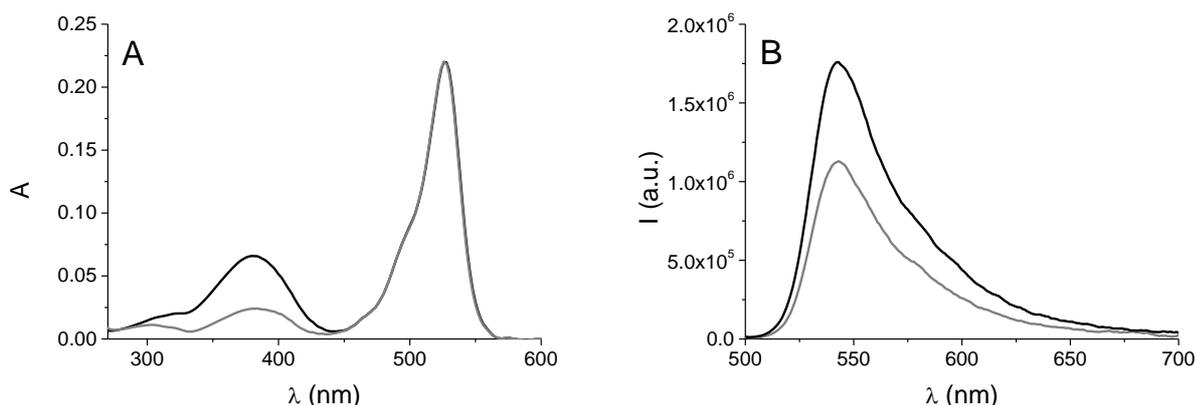
**Figure 1.** A) Absorption spectra of **1** (black) and **2** (grey) in acetonitrile. B) Fluorescence emission spectra ( $\lambda_{exc}=480$  nm) of **1** (black) and **2** (grey) in acetonitrile. [**1**] = [**2**] = 6.5  $\mu$ M.
