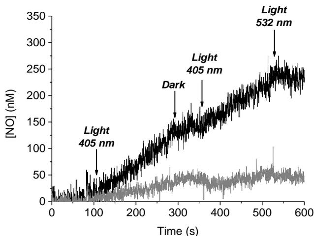
**Figure 5.** NO release profiles observed upon irradiation of solutions of **1** (black) and **2** (grey) in culture medium.  $[\mathbf{1}] = [\mathbf{2}] = 8.6 \mu\text{M}$ .
