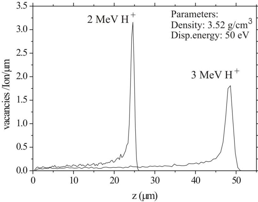
**Figure 7** Functions  $p(z)$  for implantations of protons with energies of 2 and 3 MeV.
