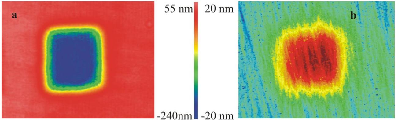
**Figure 4** a) Map of the OPD profile of an area implanted with 3 MeV protons at a fluency of  $7.5 \cdot 10^{16} \text{ cm}^{-2}$ ; b) map of the swelling profile of the same implantation. The two profiles have opposite signs because swelling gives a shorter optical path in reflection, while damage produces a longer optical path in transmission measurements.
