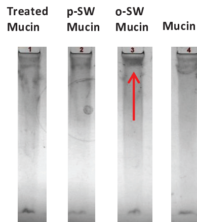
Figure 5. ND-PAGE electrophoresis of 1) mucin (control treated as samples 2 and 3 without the addition of CNTs), 2) mucin/p-SW CNT complex, 3) mucin/o-SW CNT complex, 4) mucin.
