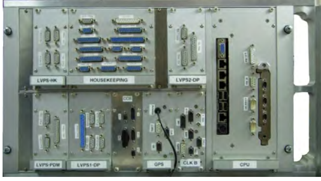
Fig. 4 The Data Processor (DP) collects and processes the data from the PDM. It handles their on-board storage, and sends a subset to the telemetry system. The DP also includes the housekeeping system. The various sub-assemblies are contained in an aluminum crate to assure thermal contact with the radiator.
