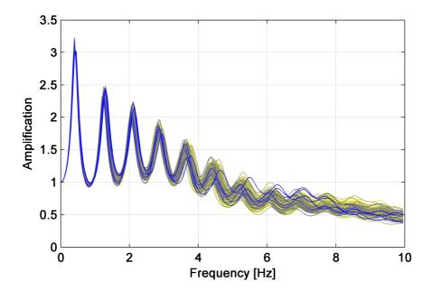
Figure 2 – Amplification functions obtained with SHAKE91 for the selected profiles in Figure 1a (Bedrock position: 150m from ground surface). The results are reported with the same color scale of Figure 1.
