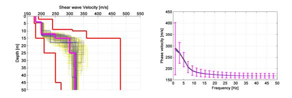
Figure 1 –Synthetic dispersion curve of case A in Boaga *et al.* (2011) is inverted with the approach of Foti *et al.* (2009): a) selected equivalent solutions compared with true model (magenta) and model space boundaries (red); b) experimental (synthetic) dispersion curve (magenta) and synthetic dispersion curves corresponding to selected models. The colours of each numerical dispersion curve is the same of the corresponding model.
