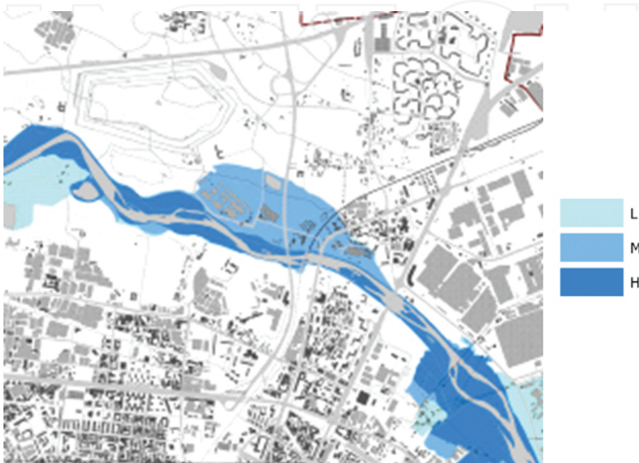
Figure 3. Flood inundation areas in Turin (free map available on Regione Piemonte website 5 ), for different flood scenarios.
