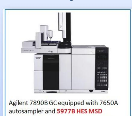
operating in El mode at 70 eV - FID detector Scan speed 20,000 amu/s Etune option
