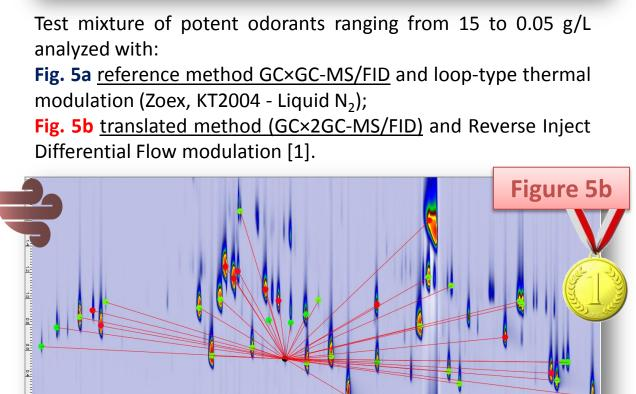
reliability guantitation (referred to as accuracy for simplicity) is evaluated taking as benchmark estimated amount (g/L) derived from FID Response Factors GC×GC-MS/FID thermal modulator arbitrarily reference considered
