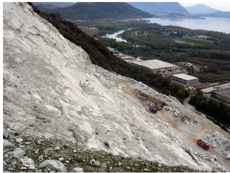
FIGURE 9: The uncovering of granite substrate thanks to mechanical equipments. The material is transported to the plant, located just below the slope (on the other side of the street).
