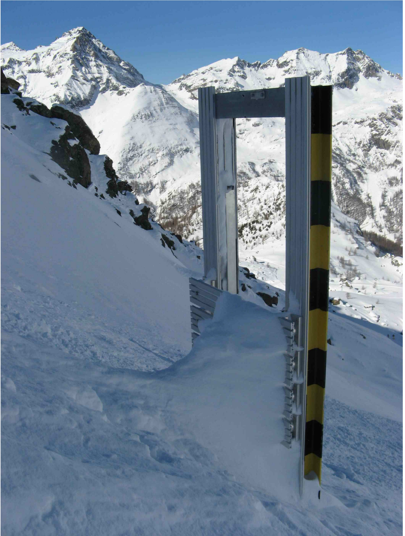
Figure 5: Detail of the load limiter device linking the two parts of the obstacle.
