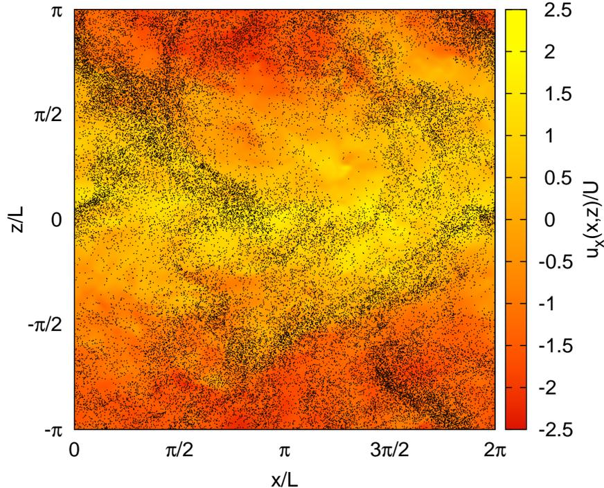
FIG. 1. Particle distribution in a slab of thickness  $2\pi L/10$ , plotted over the corresponding stream-wise component of velocity (color map, red to yellow online). Particles inertia is  $S = 7.9 \times 10^{-2}$  and  $Re = 990$ .
