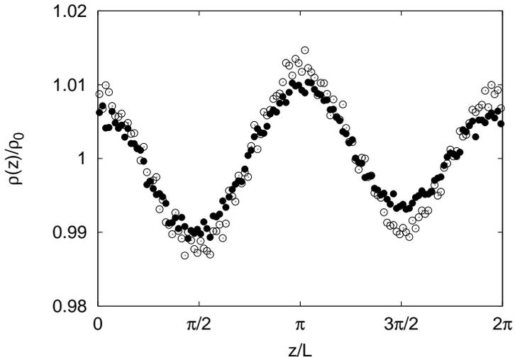
FIG. 3. Particle number density profiles  $\rho(z)$  for  $S = 4.1$  (filled circles) at  $\text{Re} = 230$ . The particle distribution is compared the prediction  $\rho(z)/\rho_0 = \langle v_z^2 \rangle^{-1} L_z / \int_0^{L_z} \langle v_z^2 \rangle^{-1} dz$  (empty circles). Statistical fluctuations are due to the slow convergence observed for large  $S$ .
