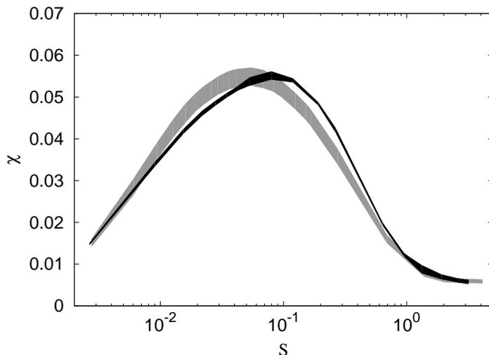
FIG. 4. Rms relative deviation  $\chi$  from the homogeneous distribution plotted as a function of  $S$  for  $Re = 230$  (grey curve) and  $Re = 990$  (black curve). The thickness of the curves reflects the statistical fluctuations around the mean value.
