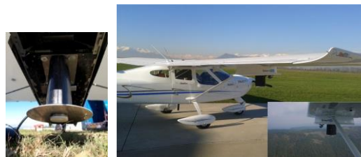
Fig. 3. GNSS-R prototype mounted on Digisky P92 aircraft.
