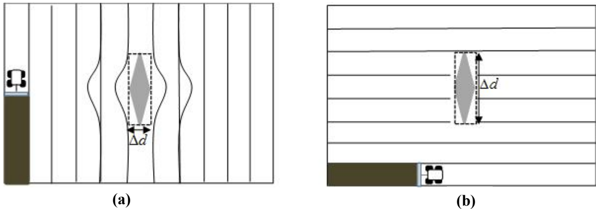
126 Fig. 3. The same obstacle can be classified as of type A (a) and as of type D (b) depending on the 127 orientation of the obstacle as compared to the driving direction where r = w .
