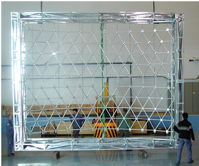
Figure 10. Picture of the mirror support structure: the nodal points are connected by light Al pipes.
