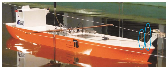
Fig. 2. Equipped model of the LNGC. (For interpretation of the references to color in this figure, the reader is referred to the web version of this article.)
