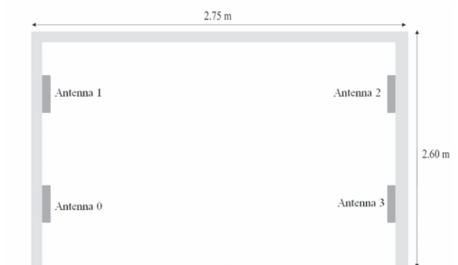
Figure 2. Gate framework: dimension and antenna position for pallets ultra high frequency electronic identification. In case of ice tea pallet only 0 and 3 antennas were used.
