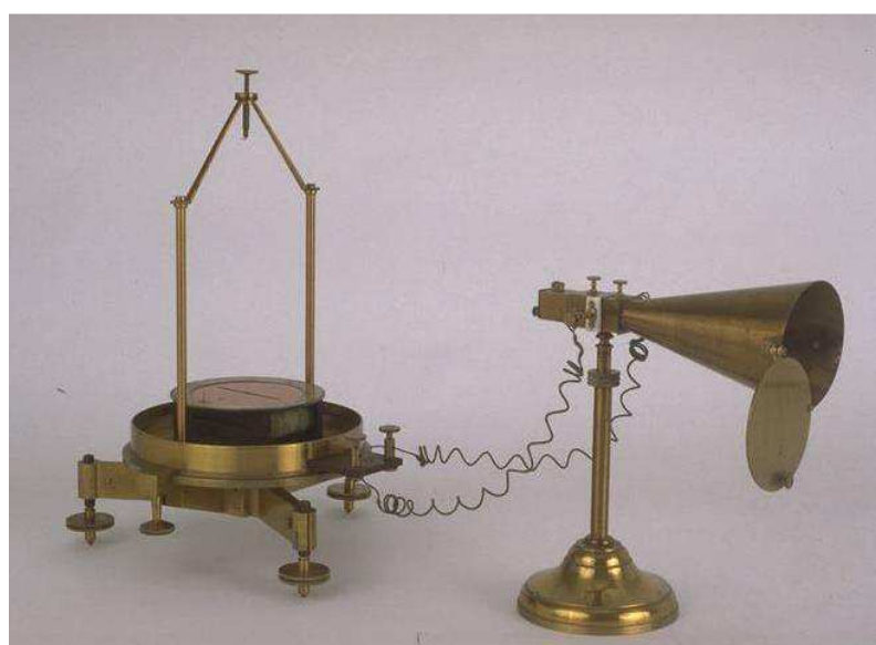
Fig. 3 – Nobili and Melloni's improved thermopile (1831) [9]
