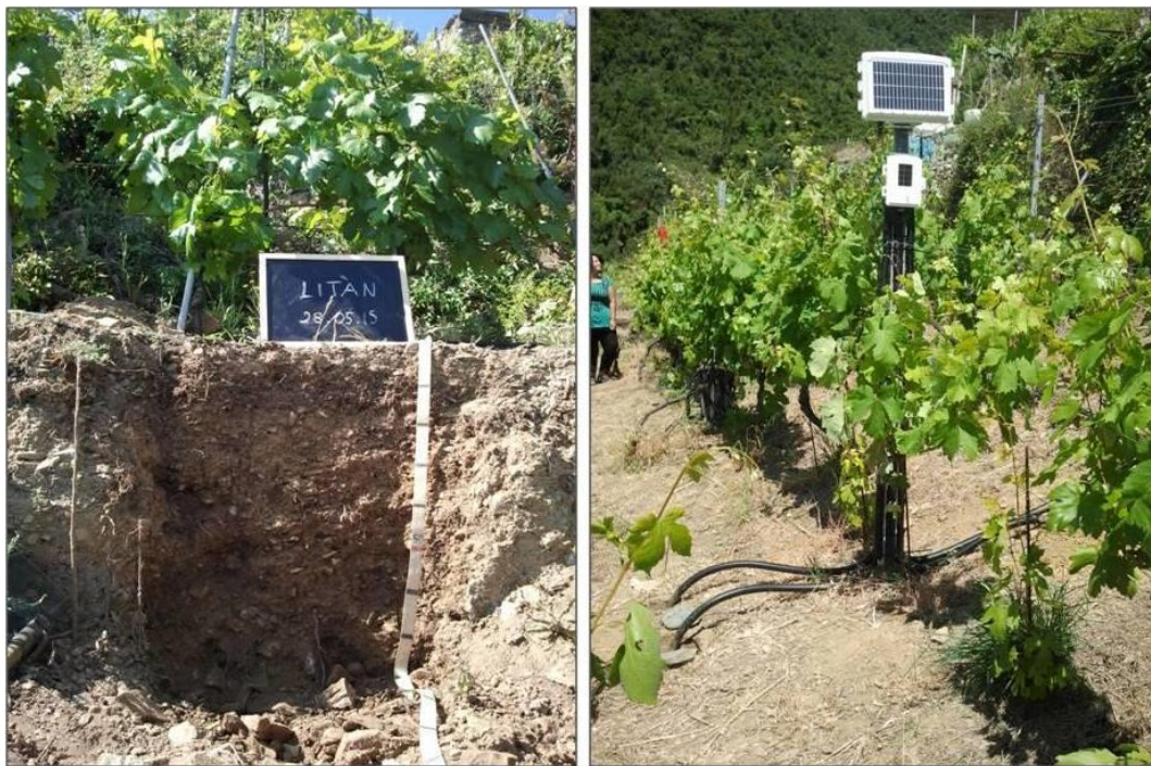
Figure 3: Views of a soil profile selected for full pedological description and sampling and of the solar-powered field station connected to multiple soil moisture/temperature sensor.
